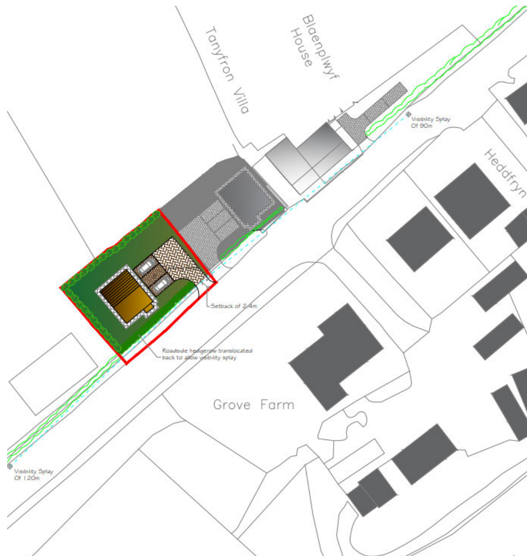
Figure 4 – indicative site layout plan of proposed replacement of farm buildings with single dwelling
