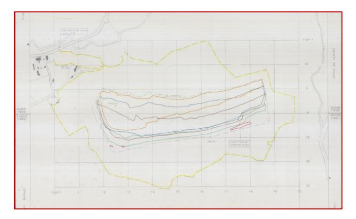
The significance of this information is twofold: This defines the area of the study site that is affected by backfilling and restoration of the ground; and also the seams that were encountered in the opencast and 'worked-out' as part of that operation.
